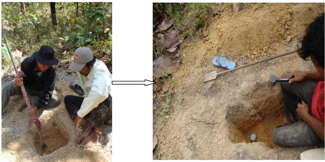
Figure 7 Soil sampling for estimating carbon pool in soil (Mondulriki province, Cambodia, 2010). Soil organic matters are included organic matter in mineral and organic soils (including peat) to a specified depth chosen by the country and applied consistently through the time series (FAO, 2007).
