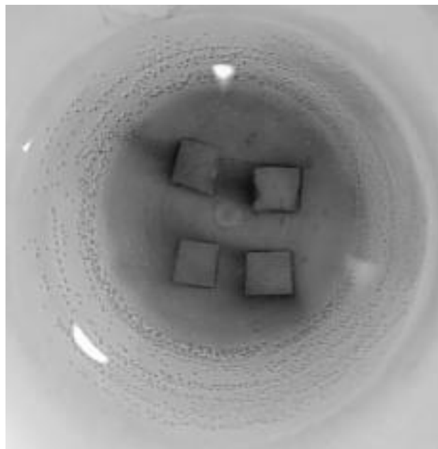
Fig. 7. 17. Photo of Si wafer in deposition solution after immersed for 3600 s.
