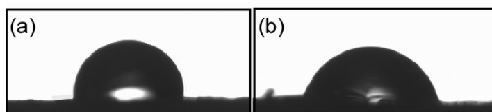
Figure 5.2.3. Water contact angles of the pellet surface of (a) SP before UV irradiation and (b) MC after UV irradiation.
